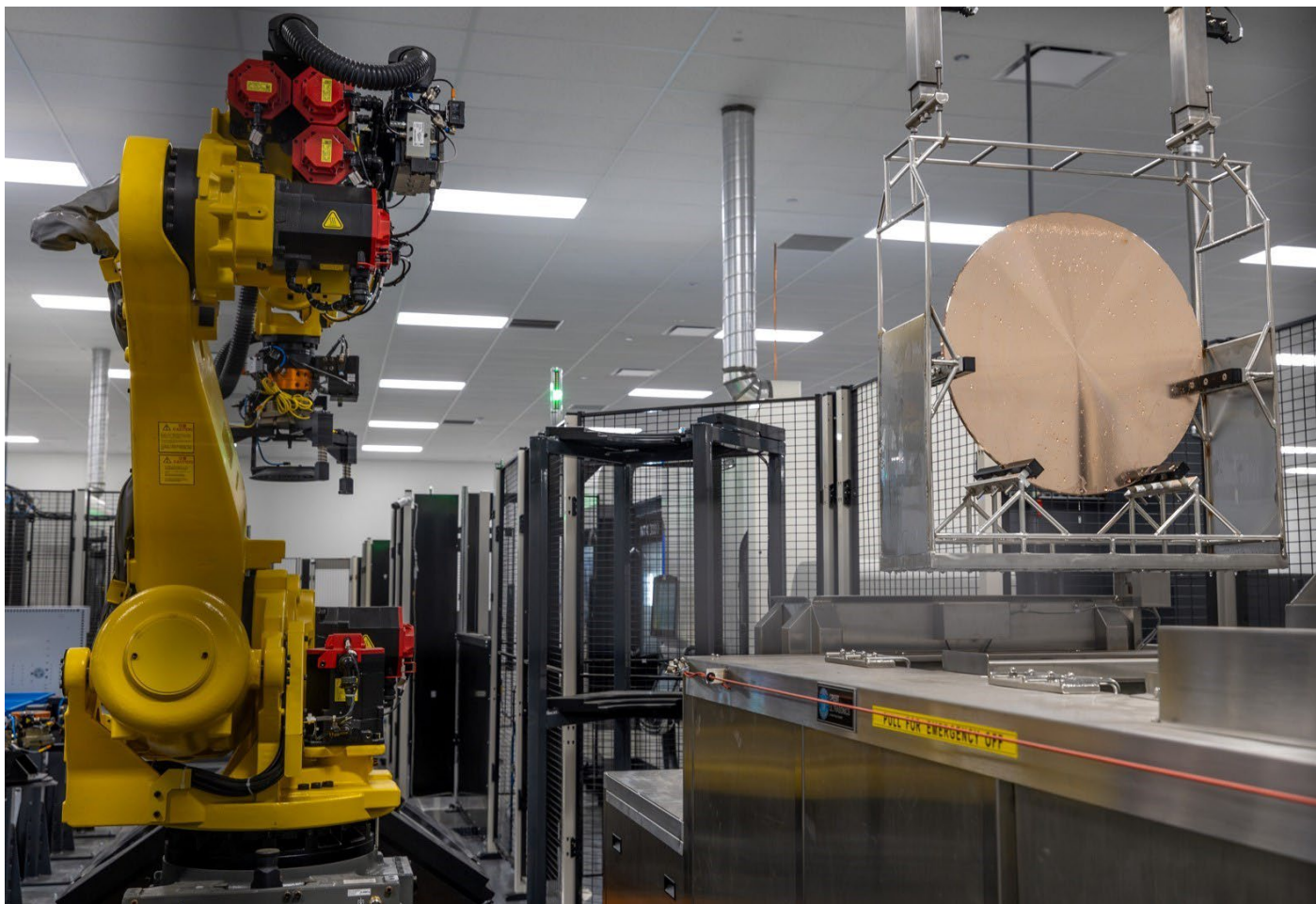
Sputtering targets are transported to the cleaning process by automatic loading equipment
