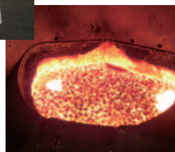
Charcoal preventing oxidization during copper processing
