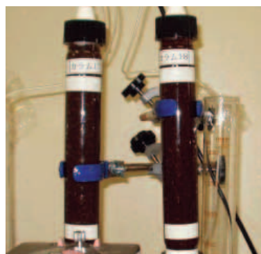
Column purification experiment to treat water contaminated with heavy metals
