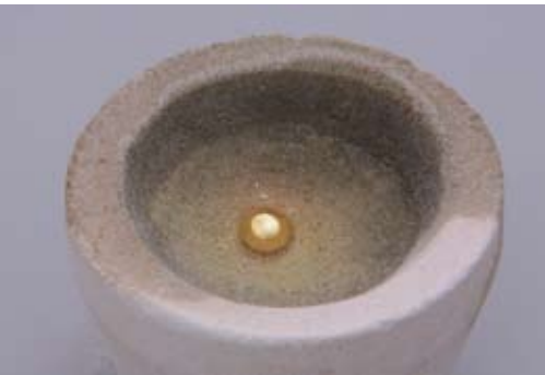
Gold bead obtained by fire assay analysis method
