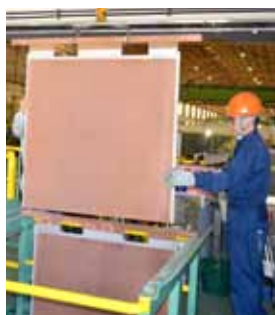
Stainless steel cathode plate with copper deposited on the surface
