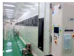
Electroless UBM plating line at Longtan Works
