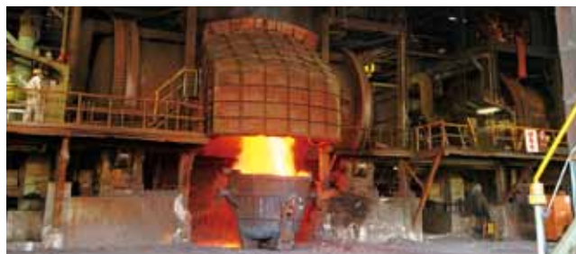
Recycling process (converter furnace) at Saganoseki Smelter & Refinery
