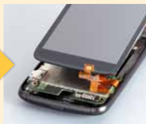
Applications: Flexible printed circuit boards
