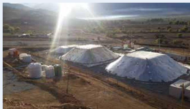
Heap-leaching experiments in Chile to verify the JX-iodine process
