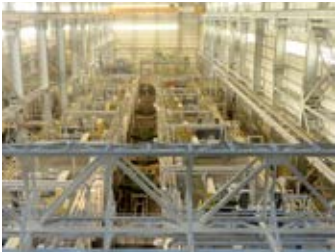
Flotation A process in which ore that has been ground in the SAG mill is separated into copper concentrate and tailings.
