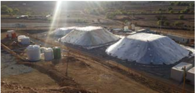
Heap-leaching experiments in Chile to verify the JX-iodine process
