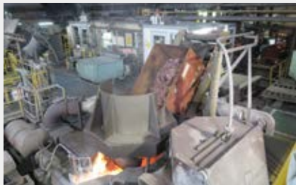
Cut copper put in melting furnace along with zinc for forming into red-brass ingots
