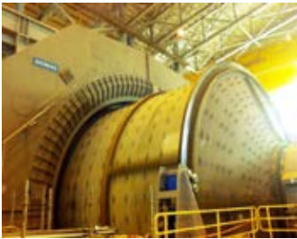
SAG (semi-autogenous grinding) mill After being crushed to 200 mm or smaller in crushing equipment, the ore is reduced to around 0.2 mm in the grinding process.
