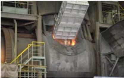
Discarded mobile phones are put into a converter furnace
