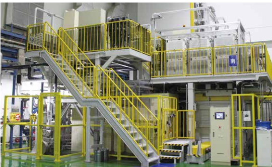
Melting furnaces, equipment used for semiconductor-use sputtering targets (Isohara Works)
