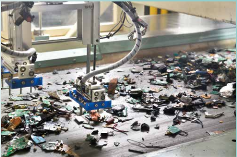
Physical sorting equipment (HMC Department, Hitachi Works) Leveraging IoT and AI to increase treatment of recycled raw materials
