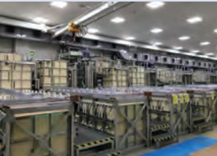
Production equipment used for semiconductor-grade sputtering targets such as electrolysis baths (Ishihara Works)
