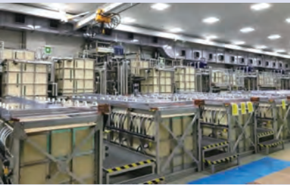
Production equipment used for semiconductor-grade sputtering targets such as electrolysis baths (Isohara Works)
