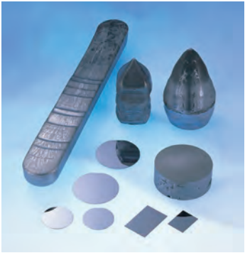
Compound semiconductor substrates (indium phosphide, cadmium zinc telluride)
