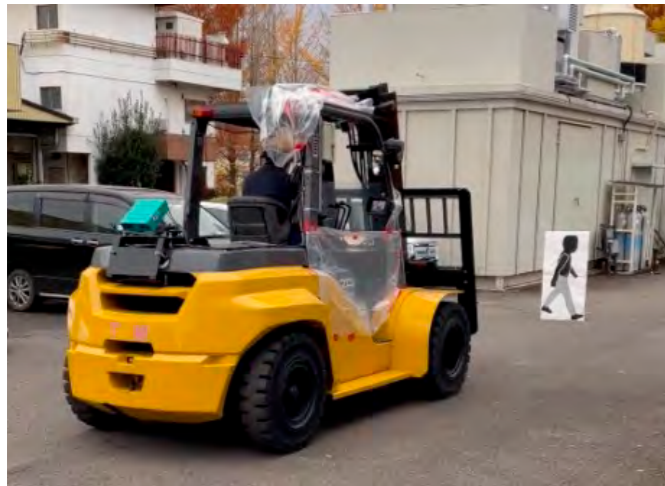
AI cameras are positioned in all directions to detect humans, strengthening and making safety measures more reliable
