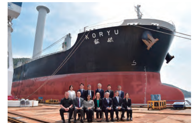
The KORYU after the installation of rotor sails
